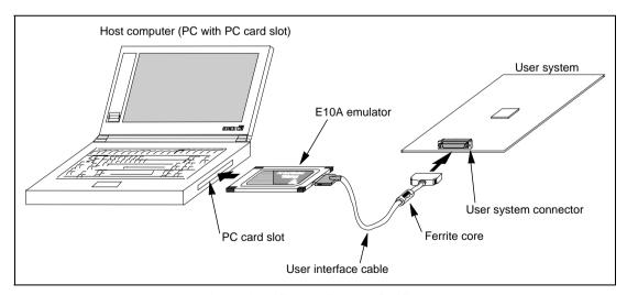
Figure 1.1 Connecting Ferrite Core
